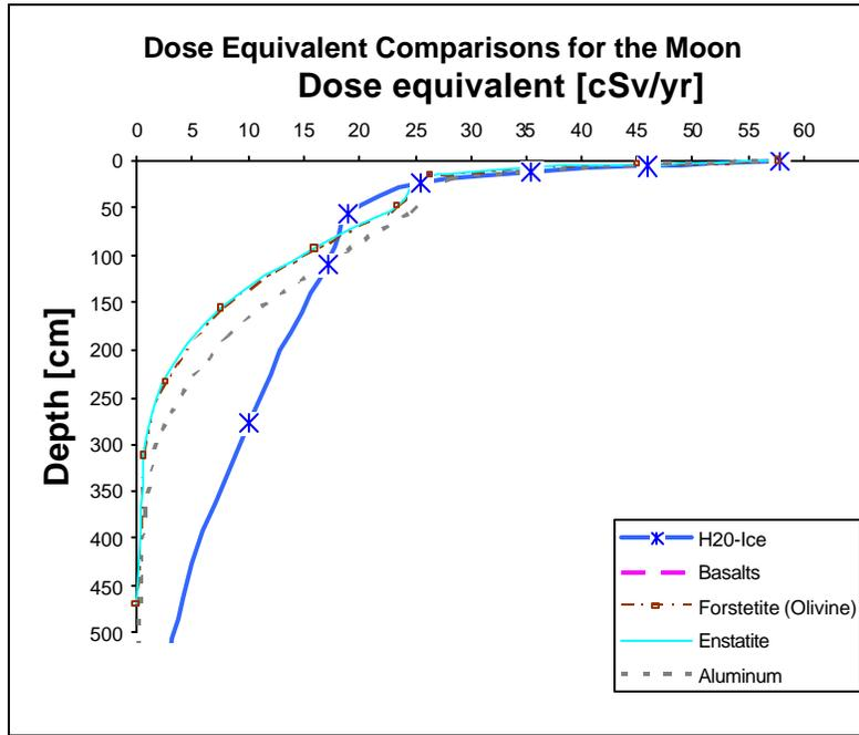
Fig 1. Comparison of radiation depth profiles for different in situ materials of potential interest on the Moon including Aluminum for a radiation scenario at Solar Maximum.
