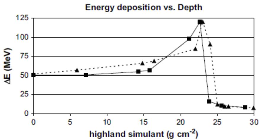
Fig 3. Energy deposition in a 3mm Silicon detector for a 290 MeV/nucleon <sup>10</sup>B beam after passing through a lunar regolith simulant. This simulates an average energy for SPEs as well as primary GCRs. [Ref.4]
