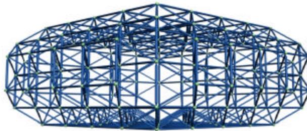
Figure 5. Internal hybrid structure for the lunar habitat.
